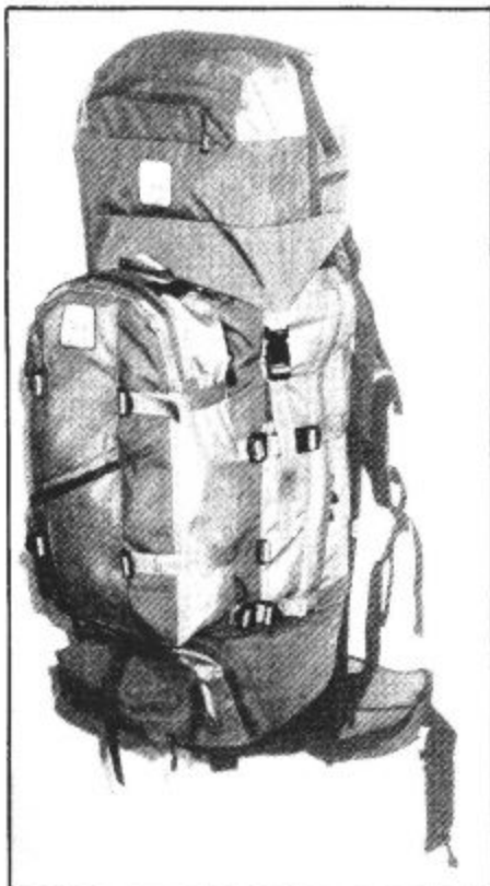
The Hamel Backpack: about 5000 cubic inches and 6 pounds, made of 500d Cordura. Includes daypack with its own suspension and detachable toiletry pocket. Top pocket has three separate compartments. Top loading and zipper side access; separate sleeping bag compartment with zip-out divider. Suspension is twin 1-inch aluminum stays plus Delrin rod.
